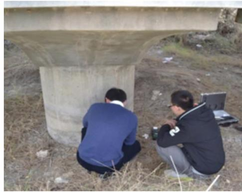
Fig. 5. Hardness test of pier
