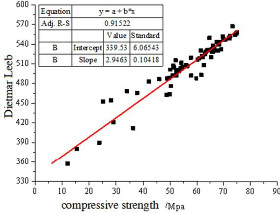
Fig. 3. The fit map of Concrete hardness and strength
